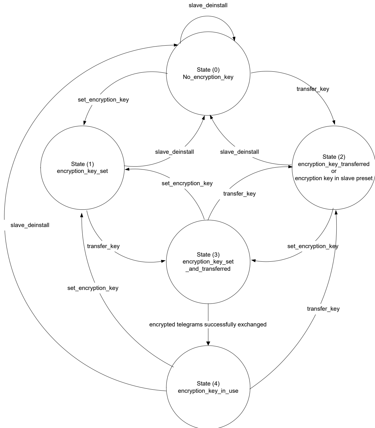
Figure B. 1 – Encryption key status diagram
