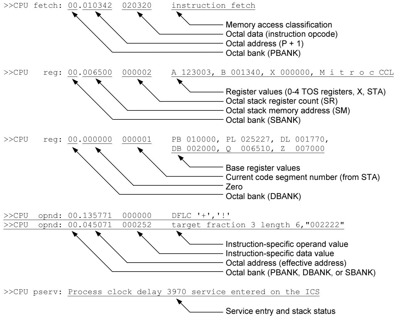
For **OPND** traces of byte-array operands, the data values printed are the relative byte addresses. For **EDIT** subprogram operations, the value of the loop counter is printed.
